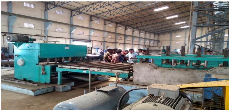
During the visit students viewed various sections in HMIL like- Press Shop: In this a computer-controlled line converts the sheet metal to body panels with high dimensional accuracy and consistency.
